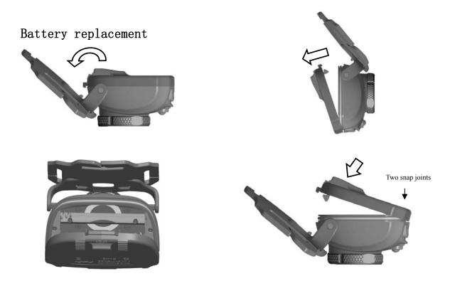
1 Pull the headlamp bracket open as the arrow indicates till it is separated from the base as shown above .
