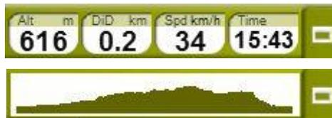
Data bar can be configured from 'menu > settings > display > Data bar'.
