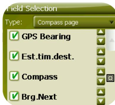
5. You may modify the order of the data on screen with the arrows on the right of the window and they will shift the datum up or down one position.
